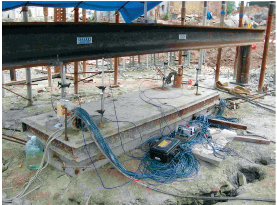
This setup was for a 10,000 ton (88 MN) test on a barrette in St. Petersburg, Russia
